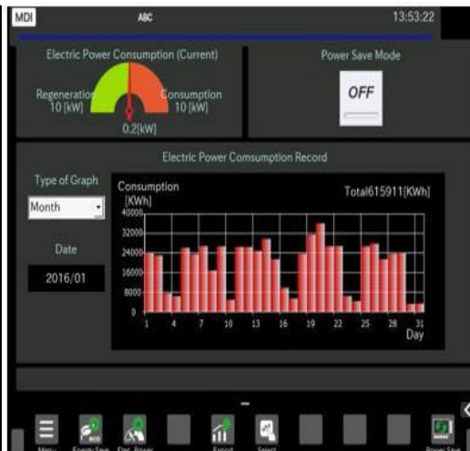
Energy consumption and saving display in machine through regenerative method
